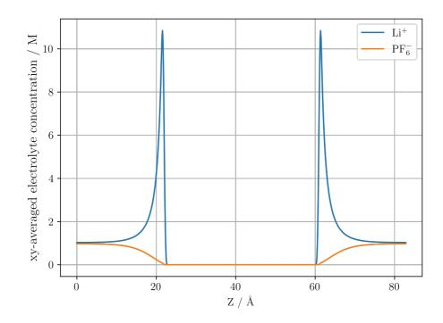
Looking at the figure above we can see that the concentration of the lithium electrolyte species is highest (12M) at the surface of the electrode, and decreases as we move away from the surface, forming a double layer along our surface. In contrary we can observe the PF6 electrolyte species has a concentration approaching 0M at the surface, and increases as we move away from the surface, note that these are local concentrations and not bulk concentrations.
