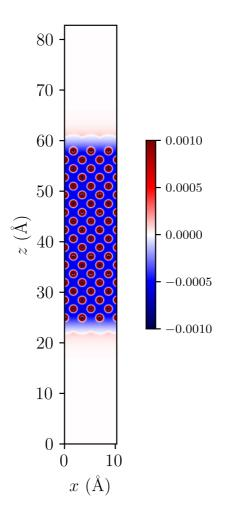
Here we can see that there is a positive charge denisty (our lithium ions) at the surface of the electrode, that diffuses in intensity as we move away from the surface.
